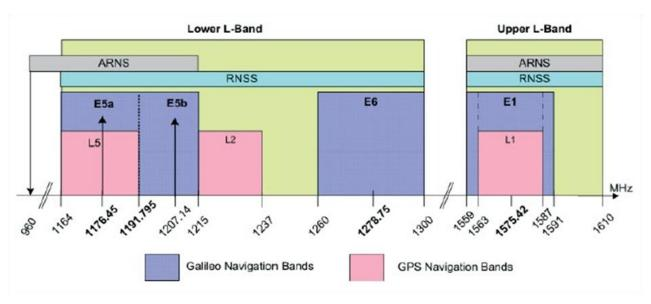
Galileo has several downlink bands. Unlike GPS, Galileo sub-band E6 encompasses 23cm.
